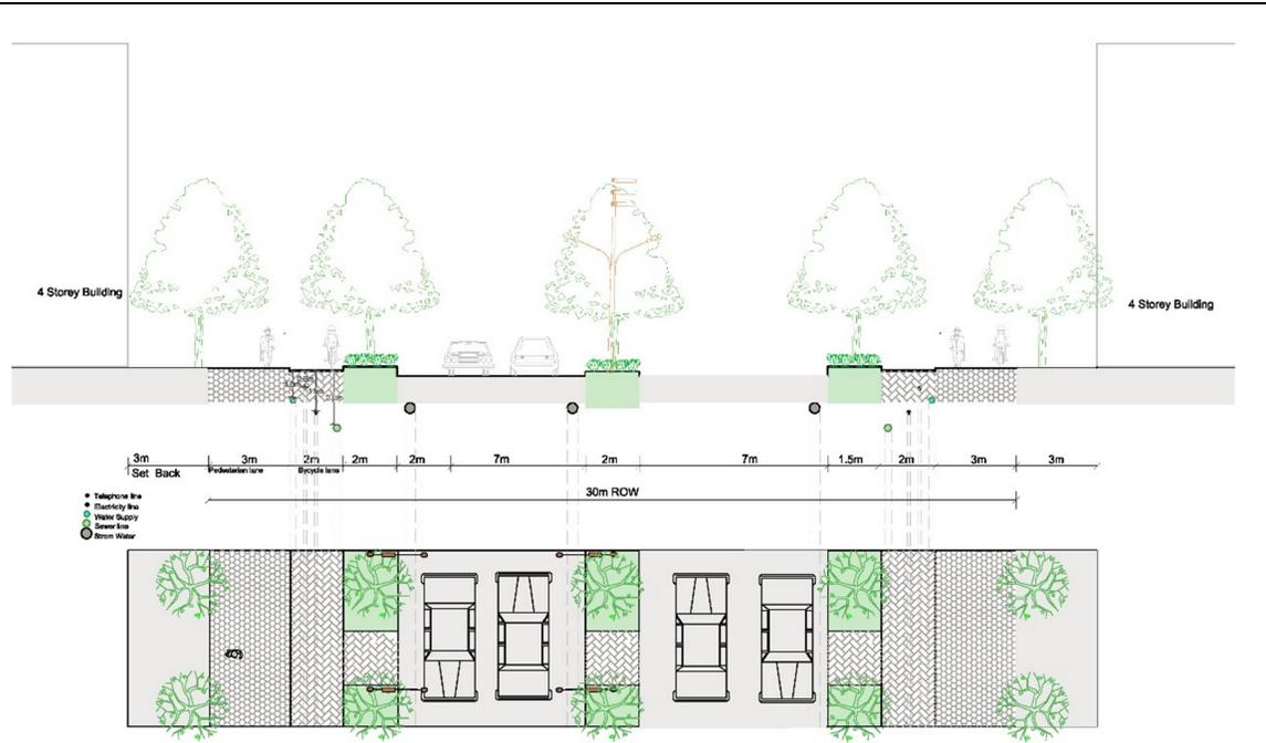
**Fig. 4.32 b Proposed road section of ROW = 30 m within city area**
