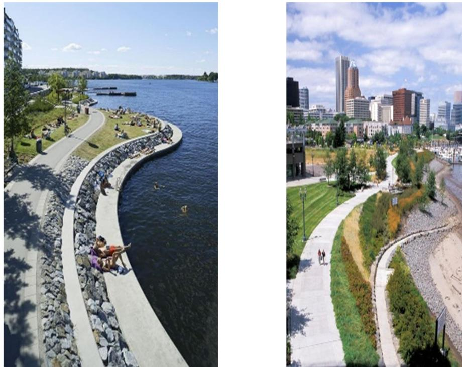
**Fig. 4.15c** Typical Bank protection between flood channel and buffer
